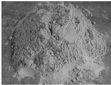
Figure 2–RHA sample after 30 minutes of grinding.
